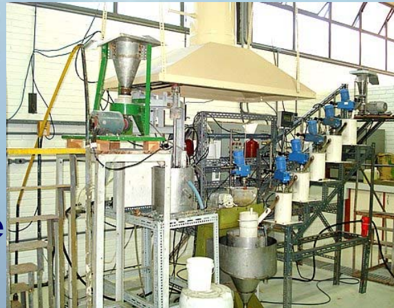
Leaching and precipitation system
